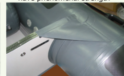
Marine-ply transom, 40 mm thick, is protected by a stainless-steel plate. Lifting holes on the transom are reinforced by stainless-steel tubes
