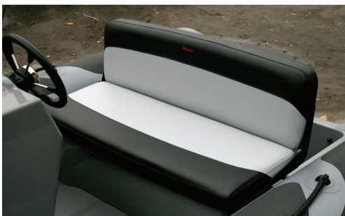
SLS-3 Soft seat for 3 persons (V-550) with internal stowage and soft backrest Dimensions, cm: (L x W x H) 124 x 60 x 82 SLS-5 Soft seat for 3 persons (V-610) Dimensions, cm: (L x W x H) 135 x 63 x 82
