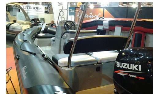
SLS 5SL soft seat for 3 persons with internal stowage and soft backrest, navigation arc and lights. Dimensions,cm (L*W*H): 135*75*140
