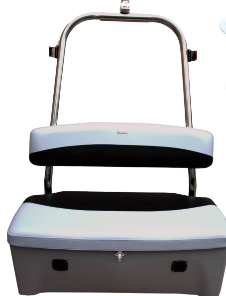
Driver Deck SLS-4 Front soft seat Stainless steel handrail Internal stowages (2 or 3 separate hermatical compartments) Dimensions, cm: (L x W x H) 82 x 58 x 91
