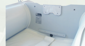
Rigid integral transom with fitted plastic plate for engine location
