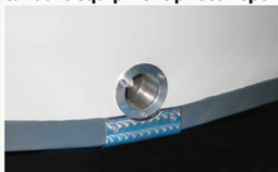
Stainless steel drain plug. Lower transom side is protected by stainless steel plate
