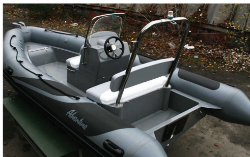
SLS-3SL Soft seat for 3 persons with internal stowage and soft backrest, navigation arc and navigation lights Dimension, cm: (L x W x H) 124 x 60 x 135 Available for: V-550
