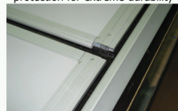
Floorboard sections are made from marine ply, of 15 mm thickness, reinforced with two longitudinal aluminium extrusions
