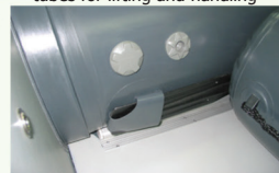
Each hermetic section of the inflatable tube is equipped with professional-series valves Leaffield (main inlet valve and overpressure valve)
