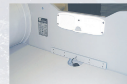
Fitted transom plate for motor, and draining plug
