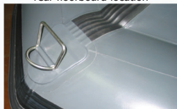
Bow handle in stainless-steel with combined towing-ring. The inflatable keel has extra protection
