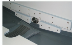
Drain plug showing stainless cap through aperture in floor
