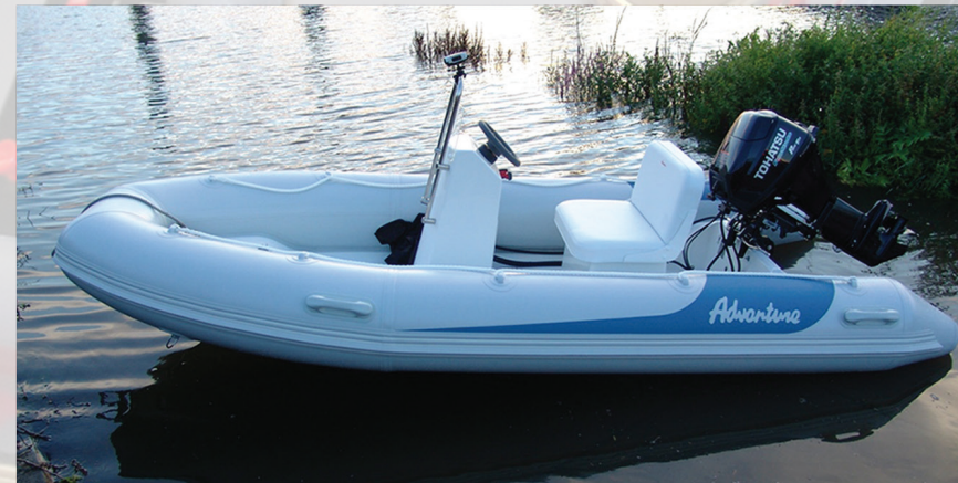
V-380 (light grey color) with ML-1 steering console, SLS-1 soft seat
